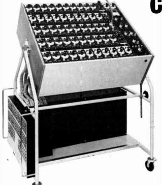
The photograph shows the 50-way trolley-mounted console of a complete sound distribution and mixing system recently completed to special order. Ideal for either studio or location work, it operates either from mains or 12 volt battery and incorporates a jack field and two integral 30 watt power amplifiers.
