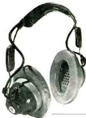
65/1B LIGHTWEIGHT STUDIO MOVING COIL HEADPHONES Omnidirectional Frequency Response 50 Hz to 15,000 Hz Impedance: 300Ω per earphone Sensitivity +45 dB ref V/dyne/cm 2 Weight 11oz. (300g.)
