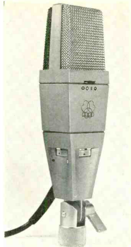
Above: AKG C414 variable pattern capacitor studio microphone.
