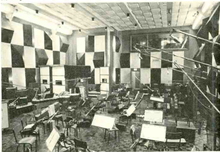
The Decca Studio A laid out for a session. The cabins are not shown. Note the acoustic treatment on walls and ceiling.
