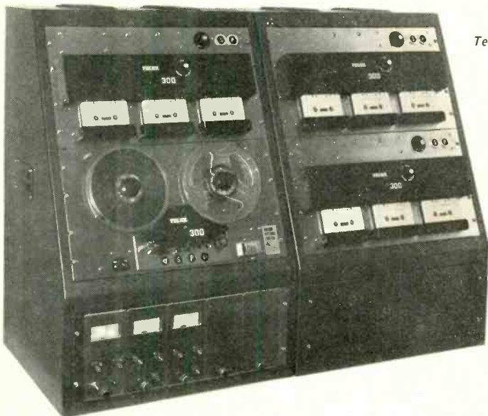
Right: BKM6 master console—part of the AEG-Telefunken range. This machine operates with two 25 mm masters providing continuous duplication at 32 times playing speed for both 8 track and cassette production
