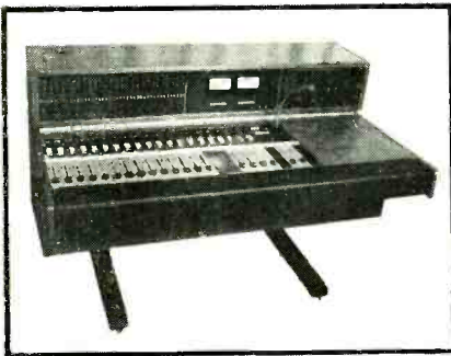
B102 14 to 32 input, 4 sub group, 2 main output control console.
