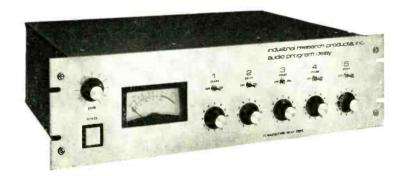
The Audio Program Delay (DA 4003) offers up to five outputs from a single input with time delays up to 240 milliseconds. Delay steps of 10 milliseconds are standard and are selected with panel mounted switches. The versatility of delay selection with multiple outputs gives the professional recording artist an opportunity to produce a variety of sound colouring effects.
