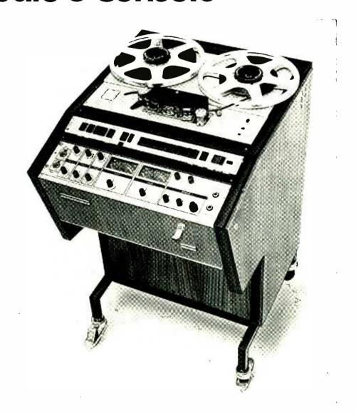
Full logic control. Tape motion sensing. Two speeds. Servo-controlled capstan. Constant tape tension. Direct-reading tape timer (minutes and seconds). Three editing modes. Provision for synchronisation, remote control and remote display panel. Available for line-in/line-out or with mixing and monitoring facilities. IEC or NAB equalisation. Full or
