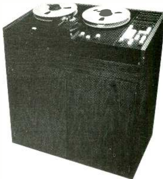
Right: The new digital tape machine from 3M handles 32 tracks on 25.4 mm tape.
