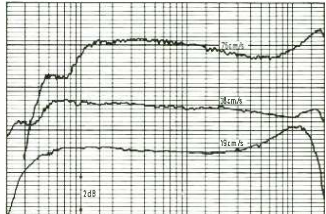
FIG. 3 OVERALL FREQUENCY RESPONSE ZERO LEVEL: -10dB ref 200nWb/m
