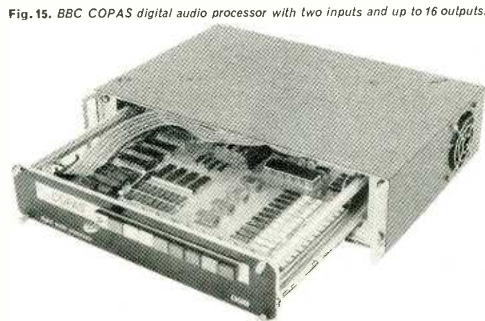
Fig. 15. BBC COPAS digital audio processor with two inputs and up to 16 outputs.
