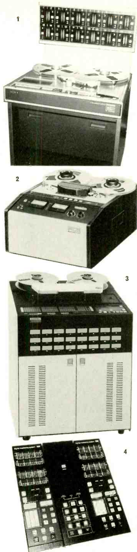
1, Sony digital 24-track, 2, Mitsubishi digital 2-track, 3, Ampex 24-track ATR-124, 4, two 3M digital remote controllers with editor in centre.
