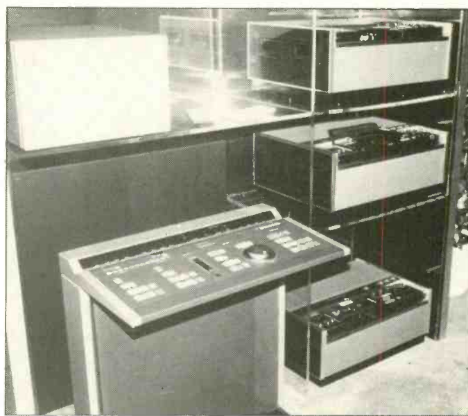
Above, Soundstream 4-channel digital tape recorder using standard instrumentation tape recorder with digital adaptor (only available for hire), as used by Fleetwood Mac for Tusk. Left, Sony PCM-1600 digital system using U-Matic video cassette recorders (background), PCM adaptor (top left) and editing controller (foreground), as used by Stevie Wonder for The Secret Life of Plants.
