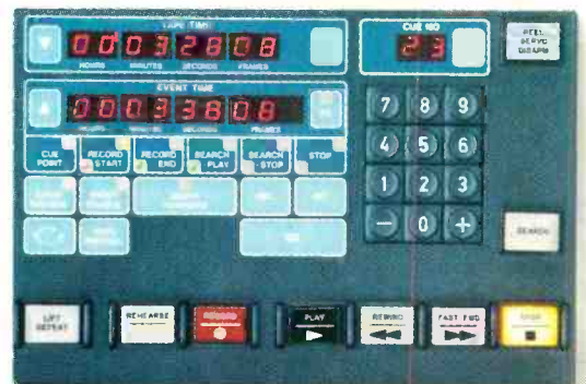
ATR-124's Multi-Point Search-To-Cue (MPSTC). Provides 100 cue locations.
