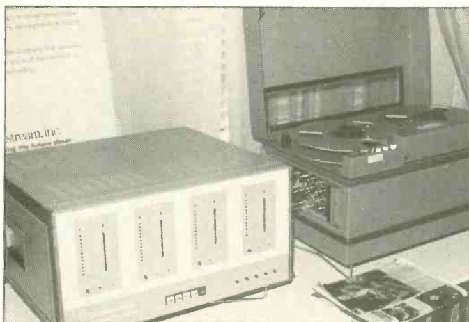
Above, Soundstream 4-channel digital tape recorder using standard instrumentation tape recorder with digital adaptor (only available for hire), as used by Fleetwood Mac for Tusk. Left, Sony PCM-1600 digital system using U-Matic video cassette recorders (background), PCM adaptor (top left) and editing controller (foreground), as used by Stevie Wonder for The Secret Life of Plants.
