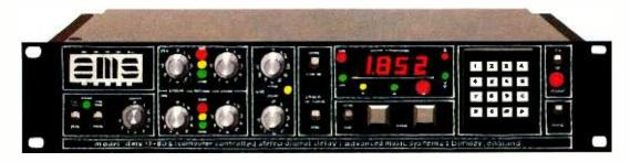
It's unusual that a piece of studio outboard equipment can be used as a creative musical tool. The Syco AMS package is now one such tool. It includes a four octave music keyboard which can be used to transpose anything stored in the "lock-in" memory up or down two octaves. Effectively this allows you to use the 15-80S package as a monophonic sampling keyboard with a bandwidth of 20-18khz and a maximum sample time of 30 seconds.
