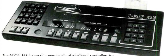
The I-CON 16S is one of a new family of intelligent controllers for audio tape and video which includes not only all the autolocate functions of the CM50 but also a choice of 16 or 24 track select keys with a serial data link to the tape deck (we provide the decoder). The 'S' suffix means that the I-CON may also be equipped as a simple synchroniser for some tape machines (including the B16 and Tascam 58).
