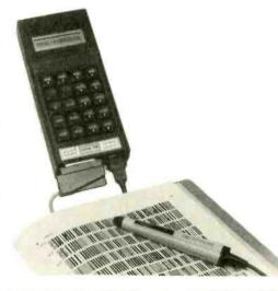
control of the RMX 16 using a normal jack cable. Secondly the remote terminal can store up to 99 user programmed settings in its own non-volatile memory allowing disconnection from one mainframe and transferrence of preset data to a second mainframe. By adding additional software to the remote terminal it is possible to connect a bar code wand and A.M.S. are already supplying new programmes for the RMX 16 in the form of sheets of bar codes.
