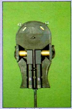
Going under the name of KU 81 the latest dummy head developed by Neumann contains two capacitor mic amps. The ear is made of material which has very similar mechanical properties to human flesh
