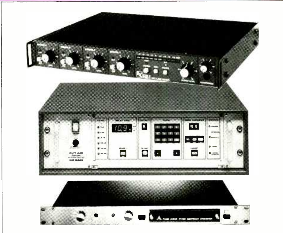
Top to bottom: E-V ELX-1 mic/line mixer, EMT445 digital audio delay, FM Acoustics FM230 linear phase electronic crossover
