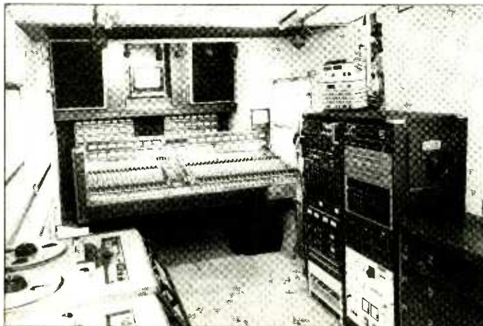
The automated custom Raindirk console is loosely based on the 500
