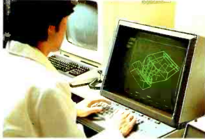
Computer simulation of the acoustic characteristics of auditoriums
