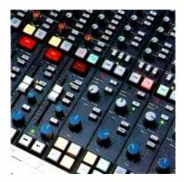
Consider, for instance, that only SSL has builtin track remotes on every channel, integrated with the industry's most versatile monitor fader and foldback facilities. Or that SSL alone provides pushbutton signal processor routing for each channel's noise gate and expander, compressor/limiter, high and low pass filters, and parametric equaliser bfree audio subgrouping
