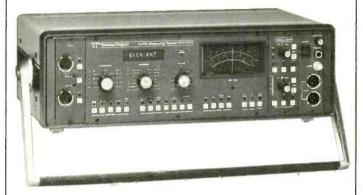
The TP401 is a high performance general purpose test instrument comprising generator (10HZ to 300KHz) and analyser (10HZ to 100 KHz), for measuring noise level, THD, IMD/TIM, W&F, cross talk and frequency.
