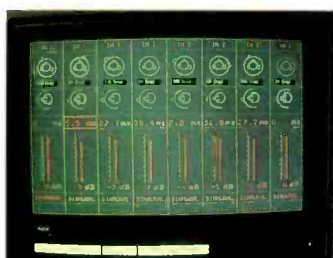
The mixer: up to 32 channels, shown here are eight binaural channels. The function framed, in this case distance to listener expressed as a function of time, is ready to be altered
