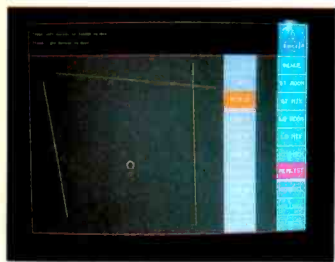
Moving walls: various walls and sound sources (channels) can be moved around the listener. The walls can be made from any material
