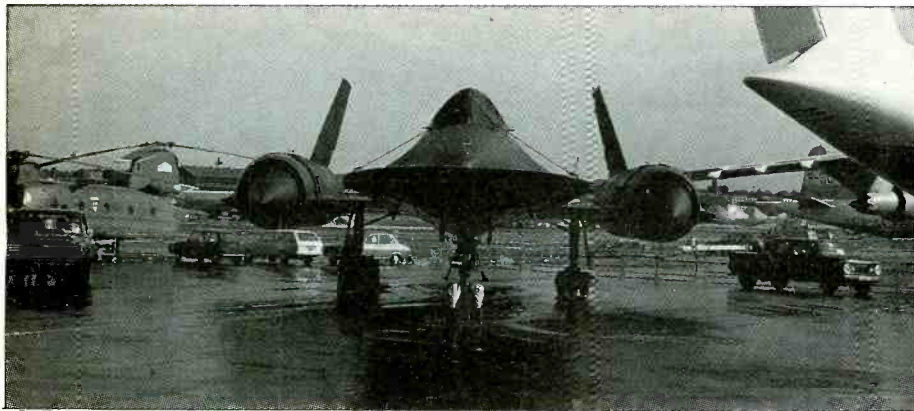
Aircraft designed for transonic speeds, comply with the aerodynamic area rule by making very gradual changes in cross-section. Thin wings gradually flatten in section at the roots, smoothly blending into a flattened fuselage cross-section.
