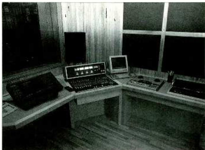
SoundStation outputs to a Studer 962 console. The A730 and Apple Mac stand in attendance
