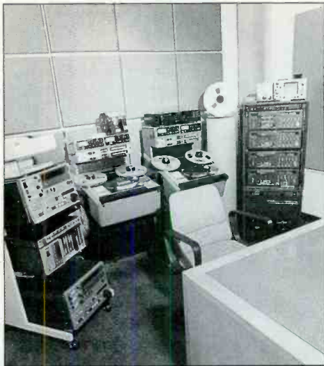
Each restoration room houses a Sonic Solutions system plus custom-designed, 4-channel monitoring console. All production rooms are interconnected via a multichannel fibre-optic network based on Sonic Solutions MediaNet
