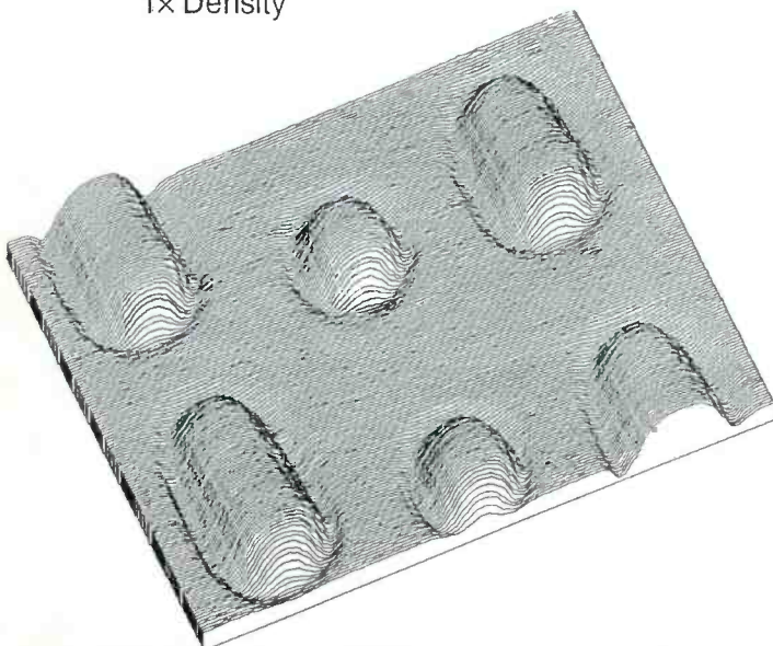
AFM Profiles of standard and ultra-high-density NPR CD masters
