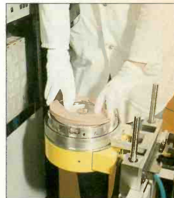
Balzers CDI 905 metallisation system needs no tools for target and mask change
