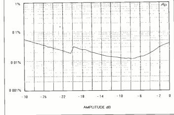
FIG 4: THD+N (30 kHz bandwidth) vs amplitude (dB re clipping) Output 1 set to 20 ms, 0 dB gain, 0 dBu headroom setting
