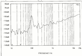
FIG 3:  $^1$ /3-octave bandwidth noise (dB re clipping) vs frequency Output 1 set at 20 ms, 0 dB gain, 0 dBu headroom setting
