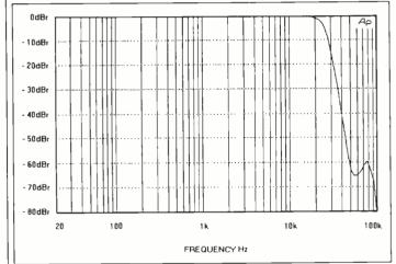
FIG 7: Output level vs frequency Wideband frequency response showing anti-aliasing filter 0 dBu input, Output 1, 0 dB I/O gain, 0 dBu headroom Delay set at 40 ms Curve typical of all settings and outputs
