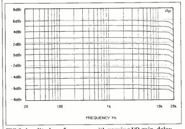
FIG 8: Amplitude vs frequency with varying I/O gain, delay set at 40 ms
