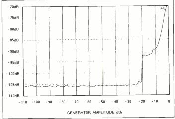
FIG 6: Quantisation distortion vs generator amplitude Headroom setting + 20 dBu Output 1 set to 20 ms, 0 dB I/O gain, 20 dBu headroom setting
