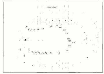
FIG 2: Wembley Stadium—delay times (ms) from west stage to loudspeaker aiming points
