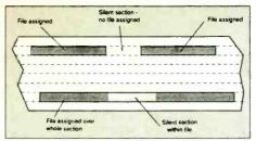
FIG 1: Two silent sections on different virtual tracks of a disk-based workstation. In the upper track the silent section uses no disk space because no recorded file exists here. In the lower section the silence has been recorded and thus consumes disk space
