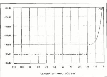
FIG 5: Quantisation distortion vs generator amplitude Headroom setting 0 dBu Output 1 set to 20 ms, 0 dB I/O gain, 0 dBu headroom setting
