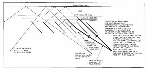
FIG 2b: Low frequency absorption in a typical trap system
