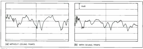
FIG 3: Effect of ceiling traps on modal pattern of room
