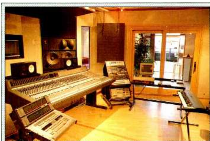
Liverpudlian Paul Downes has just opened Cavern Studios in Amsterdam. Designed by Recording Architecture, the studio features Soundtracs Quartz console and 24-track recording on two Akai DR1200 digital recorders.
