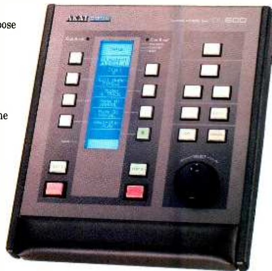
The DL600 facilitates control of the DL1000 as a cart machine
