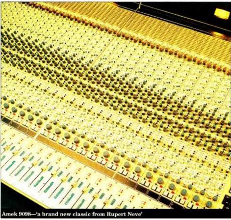
normally be bypassed. The fader block contains switches and indicators for automation, along with metering for dynamics gain reduction and channel PFL level
