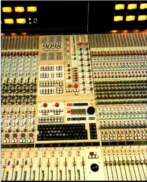
The 9098 centre section showing the considerable depth (just under five feet) of the desk and track ball for control of screen-based functions
