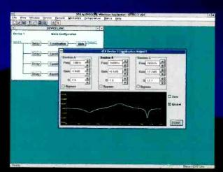
Our \*Windows™ based control software provides intuitive control over all parameters for this and future Audiocore series products, with up to 32 units controllable simultaneously.
