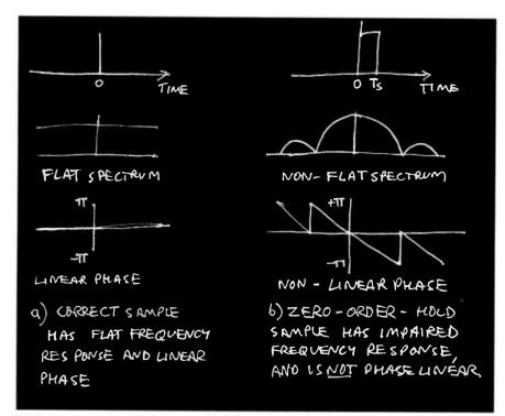
Fig.2: Correct sampling compared with zero order hold (ZOH)
