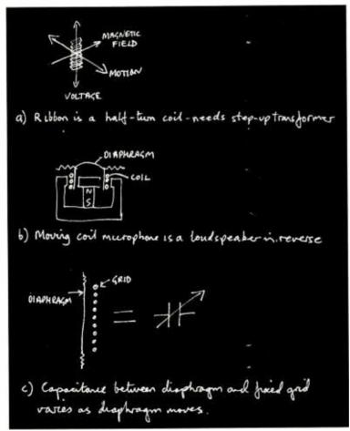
Fig.1: Microphone mechanisms
