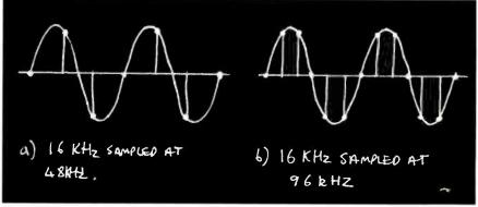
Fig.3: 48kHz is enough in a correctly implemented system
