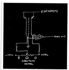
Fig.2:Variable directivity capacitor microphone adds diaphragm signals in or out-of-phase
