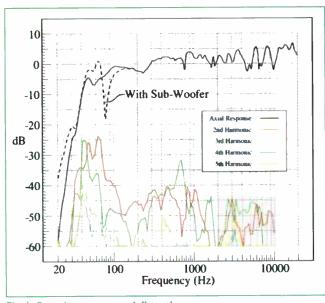
Fig. 1: On-axis response and distortion
