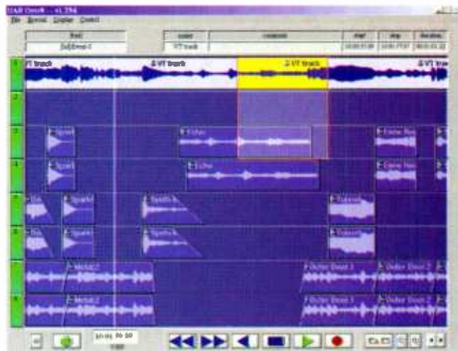
The expanded screen showing 8 tracks with waveforms and names, with a region marked for editing
