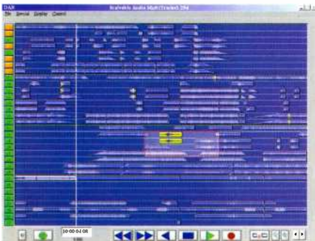
32-track display of SAM with waveforms, fades, marks, and a region outlined as editing
