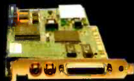
24 bit 16 Channel PCI Card (2 x TDIF as Standard)
