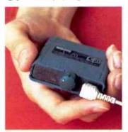
The IFB 1624 is a UHF wireless system with two channels that can be employed in sportscaster situations where split feeds are required or in a mix to mono mode giving TV presenters the ability to adjust the relative levels between two IFB sources on one earpiece.
