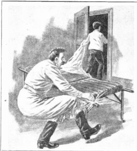
Drawing a sheet from a bed with India rubber cover thereon, produced so much static electric excitation as to give a violent shock.
