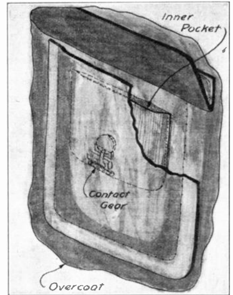
This shows the arrangement of the coin and contact pieces in the cash pocket of an overcoat.
