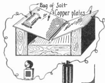
Rain alarm. The rain streaming down the copper plates and dissolving the salts, closes the circuit and rings the bell.
