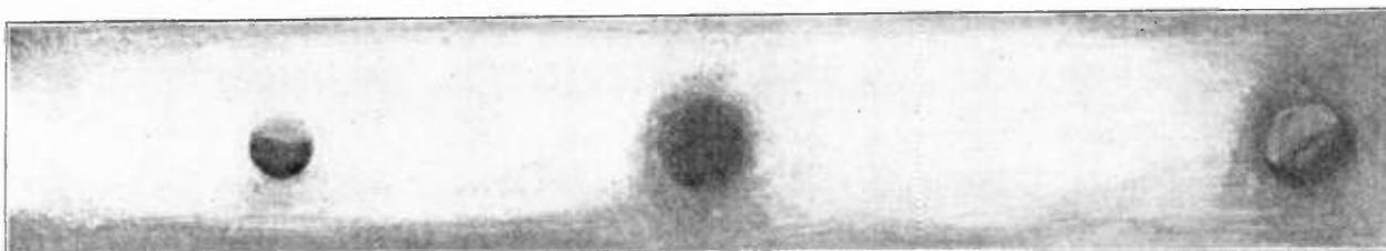
Fig. 16. Top view of the same bar. These plugs fit so well that they were indiscernible except by X-rays.
