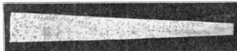
Fig. 14. A strip of copper in which the granular structure is brought out by the camera and X-rays.
