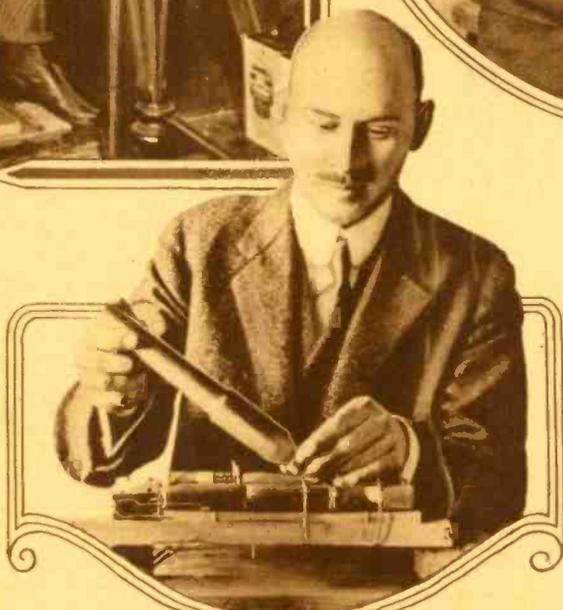
"Harnessing the electrons for heavy duty." is the keynote of Dr. Irving Langmuir's recent experiments in high power vacuum tubes, such as the 20-kilowatt tube shown above. Marconi predicts that these tubes will replace the gigantic alternators now used for long distance work.
