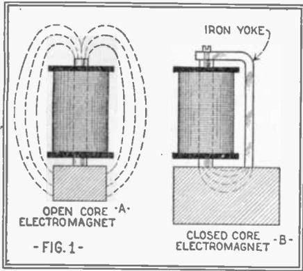
Open cored and closed cored electromagnet showing the paths of the lines of force. Observe how they vary in the two.
