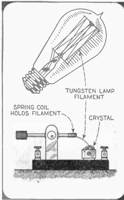
coil on the rod. The length of filament now projecting should be about one-half inch. For best results the tungsten should be bent so that it touches the crystal at right angles.
