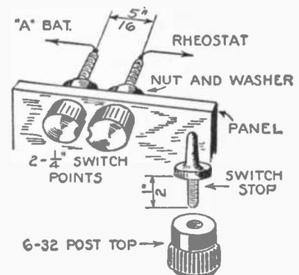
By attaching a binding post cap to a switch stop and plugging it between two grooved switch points this experimenter made a very simple filament switch.
