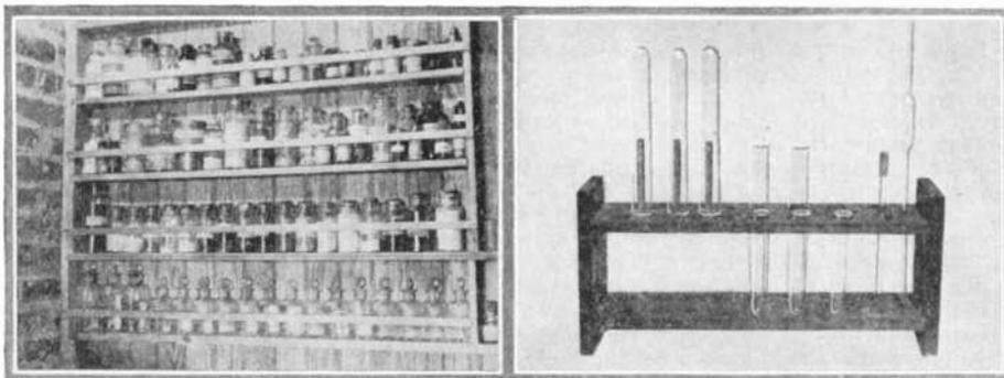
Left. A typical experimenter's chemical shelf. The guide-rails are wooden strips. The entire lower shelf is occupied by glass-stoppered reagent bottles. Right. A test tube rack can be easily made by the experimenter. Small holes in the top shelf support pipettes, stirring rods, etc. Use dowel rods for the pins.
