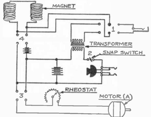
and a snap switch are mounted on the panel. They are connected as shown in the hook-up. The snap switch is the kind used in radio to cut the filament on and off.
