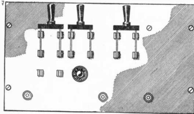
The panel board with switches of this telegraphone, designed to be constructed by the experimenter. Right—Diagram of the connections of the telegraphone, giving the entire hook-up.
