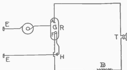
General connections of ear-phones and circuit breaker or interrupter, letters corresponding to the upper illustration. (G) is the grid.
