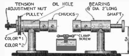
Machine for winding coils for solenoid magnets, for rheostats and the like. A very complete apparatus which will not break the wire.
