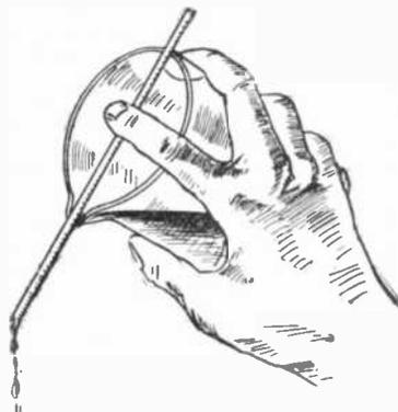
How pouring can be done with one hand. This is especially useful for small-sized beakers. For 500 cc. beakers and upward the first method is the best, and really the only one.
