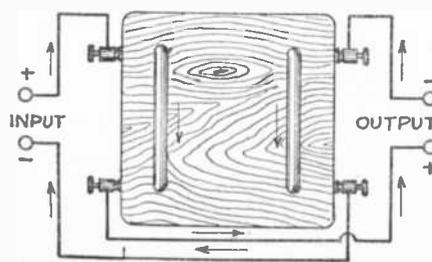
A simple reversing switch, which will prove a welcome addition to every experimenter's outfit. A sectional view of the switch, showing mercury contact wells is given; and below is shown the reversing switch hook-up.
