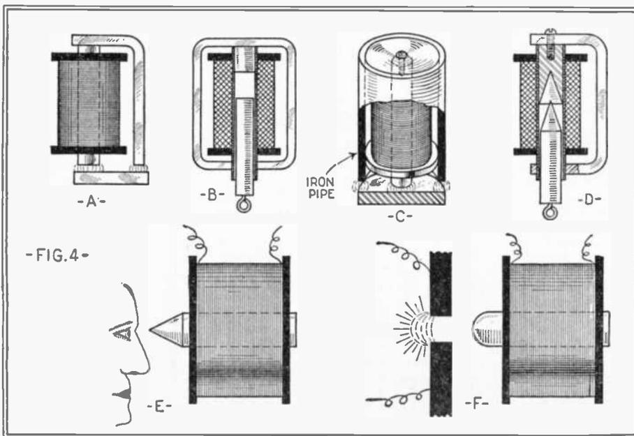
Various examples of electromagnets, including the very interesting eye magnet, which is of use in machine shops for withdrawing particles of iron or steel from the workman's eye. A jacketed magnet and an interesting example of the solenoid type may be specially observed.
