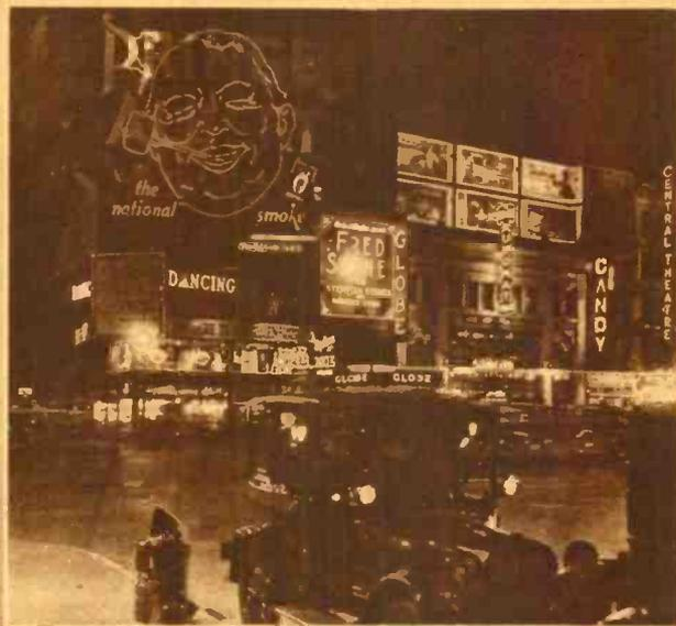
There is plenty of "ginger" in the largest electric sign on Broadway that achieves its effects at the cost of 19,000 lamps supplied through 21 miles of wire and with the consumption of over 300 horsepower. It is over 200 feet long. The jovial smoker of Prince Albert tobacco at the right is burning 2,775 electric lamps and using about 60 horsepower.
