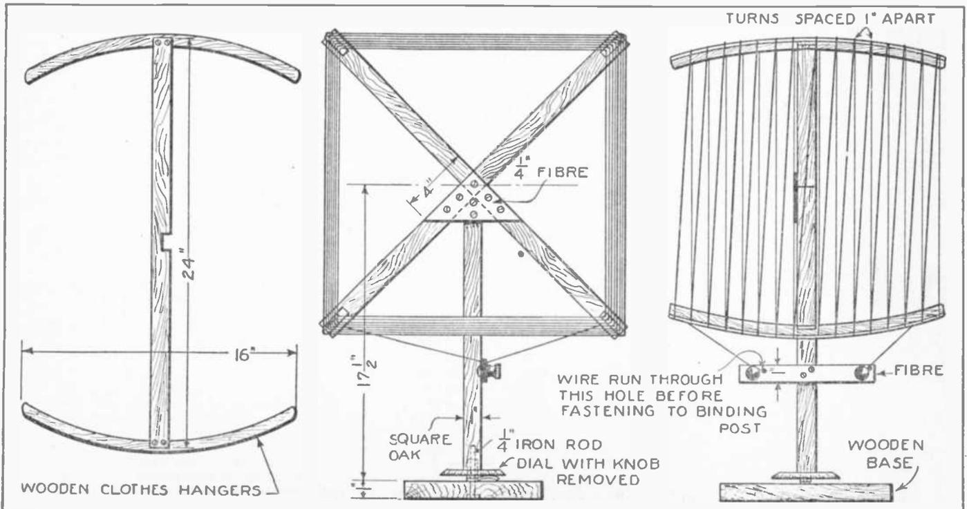
It has been observed that the slightly ball-shaped loop aerial with the turns well spaced is the most efficient type. This experimental loop is easily constructed by using four coat hangers for holding the wire.
