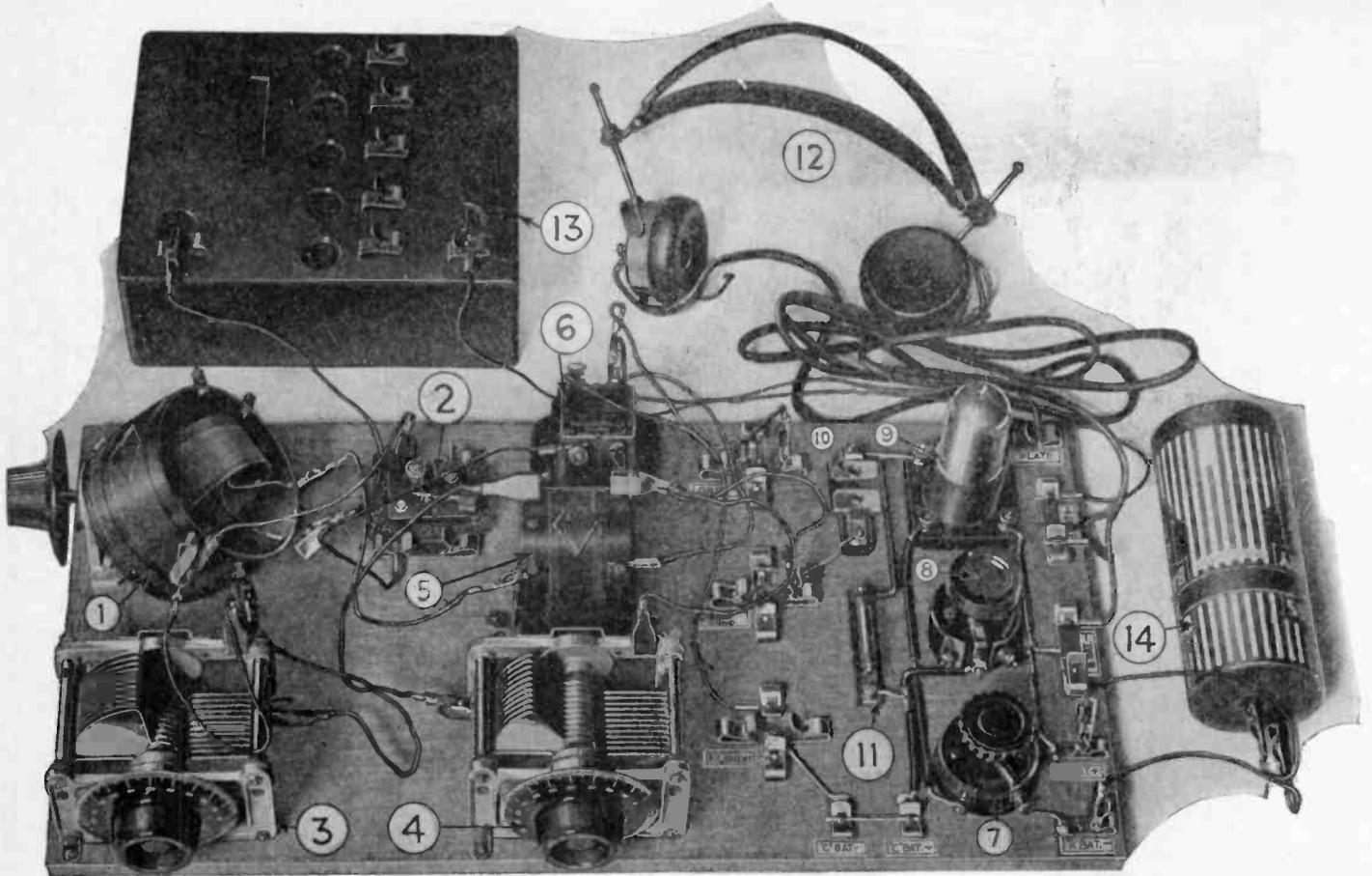
This shows how the apparatus looks after one of the experimental circuits shown on the opposite page have been hooked up. Note how conveniently the tip leads and clip leads have been applied for making the connections. In addition to the instruments mounted on the board we have (12) telephone head-set, (13) "B" battery, and (14) "A" battery. These instruments are numbered accordingly in the diagrams. This represents hook-up 6-B on the opposite page.
