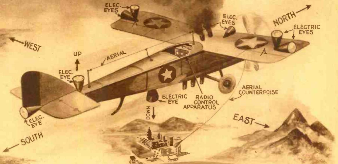
The radio television plane without a living person on board, whose movements are entirely controlled by radio from the ground. The airplane has "eyes" which look in six directions at once. Miles away from it the control operator on the ground can see what is going on around the plane much better than an aviator could even though he were sitting in the cockpit.
