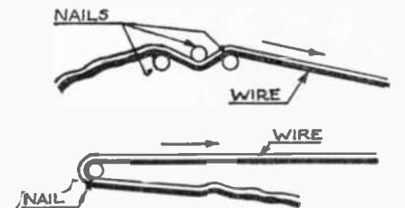
This method of straightening wires is as effective as it is simple; the three nails operate well and even the single nail will do much to improve a crooked wire.
