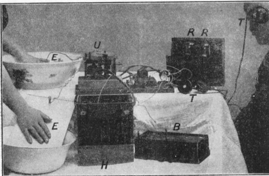
The hands are pressed on electrodes in basins of water (E, E) with a little salt dissolved in it. (B) is the battery to produce the current, (R, R) are vacuum tubes, (T) the ear-phones, (U) the interrupter mechanism, (H) the filament battery. The clenching of hands modifying the heart action gives a characteristic sound.
