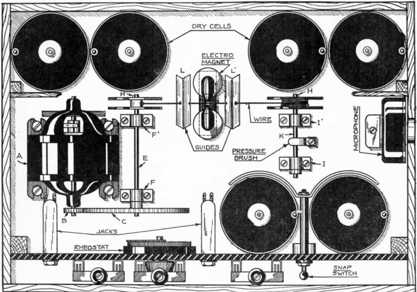
The telegraphphone, the invention of Poulsen, the Danish Edison, embodies an electromagnetic phonograph in which a steel wire represents the disc, receives the message and delivers it over and over again if desired. The wire is seen towards the upper part of the illustration, passing between the poles of an electromagnet, which impresses the message and receives it again.
