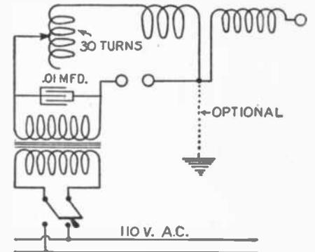
How the Tesla coil is wired, the location of the spark-gap and condenser and the optional grounding.
