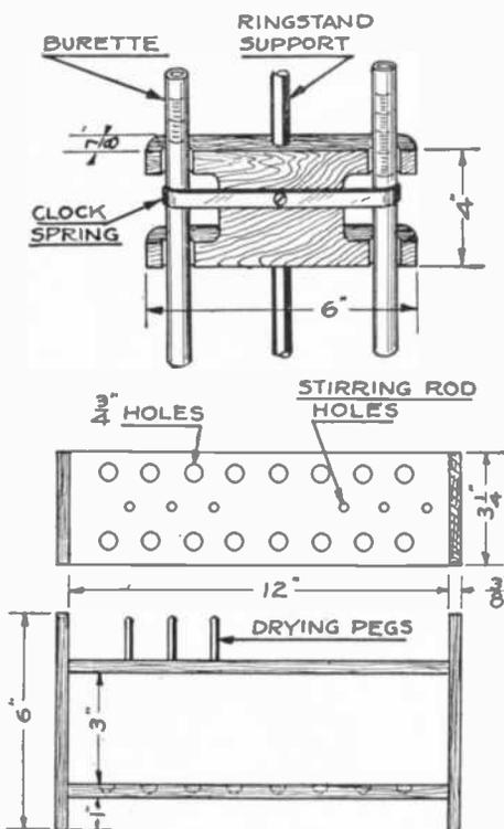
Figs. 4 and 5. A clock spring and a wooden block can also be shaped into a burette holder as shown, and below it the dimensions are given for a professional-like test tube rack which can be made from quarter or three-eighths inch wood.
