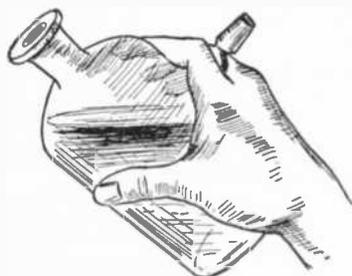
How to hold a bottle stopper when pouring out a chemical. The stopper must not touch the laboratory table, lest it should pick up impurities there.
