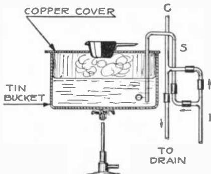
Fig. 6. A steam bath which will not burn out. A strip of paper placed in the bottom of the container will char and attract the experimenter's attention, however, if the water does evaporate completely.
