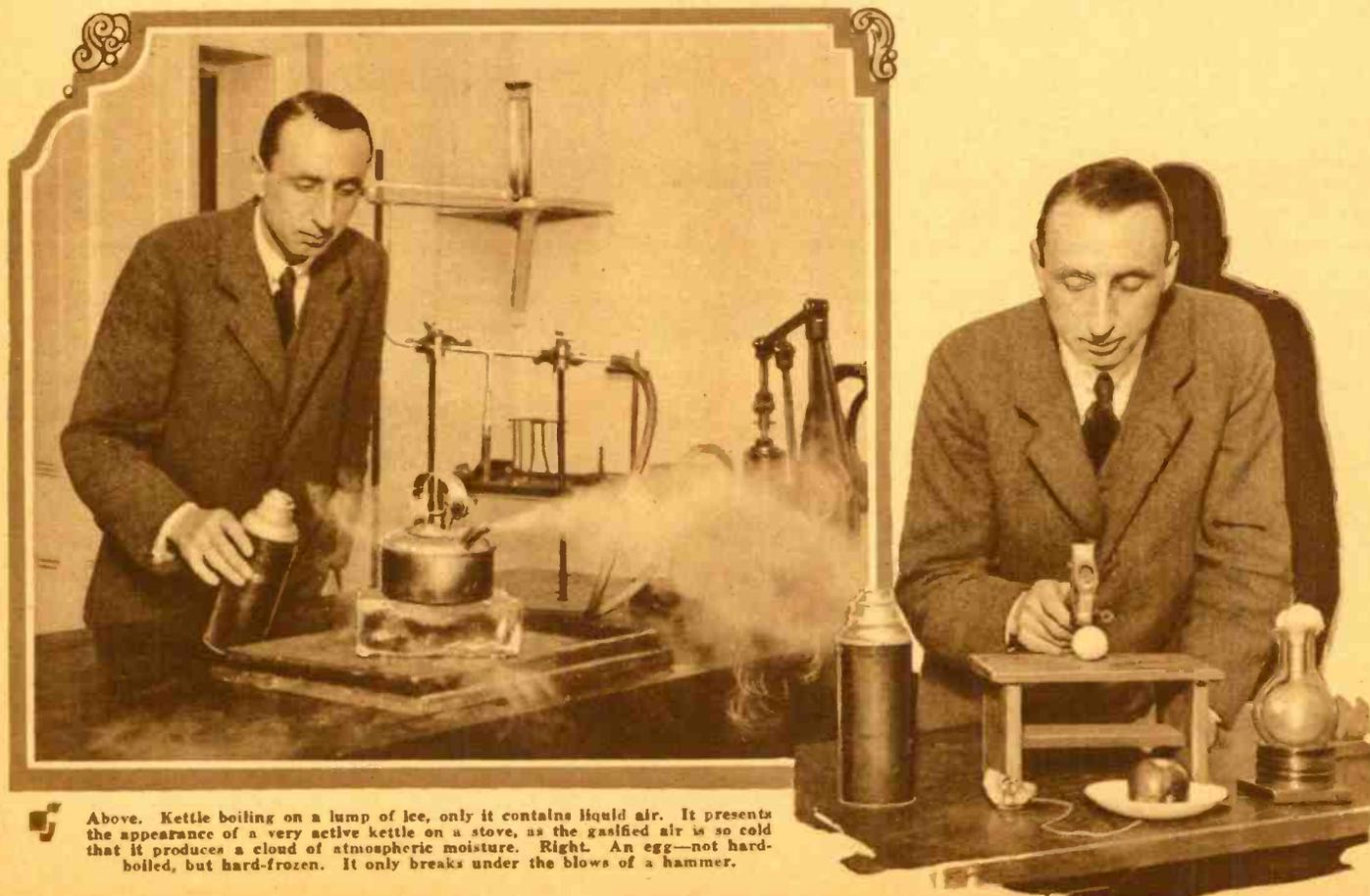
Above. Kettle boiling on a lump of ice, only it contains liquid air. It presents the appearance of a very active kettle on a stove, as the gasified air is so cold that it produces a cloud of atmospheric moisture. Right. An egg—not hard-boiled, but hard-frozen. It only breaks under the blows of a hammer.
