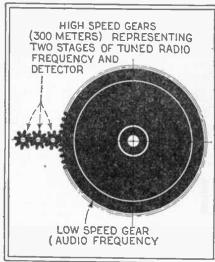
In this analogy the small high-speed gears represent two stages of tuned radio frequency amplification and detector. Note that wherever there is a change in the size of the gears detection occurs.
