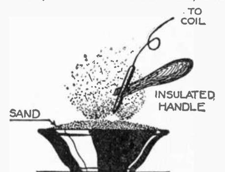
Try this spectacular eruption caused by a spark from a Tesla coil; the discharge causes sand to fly about as by a miniature lightning stroke.
