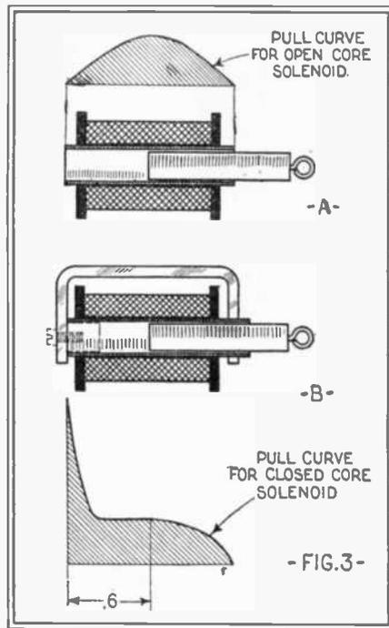
Curves of solenoids, both open core and closed core types.
