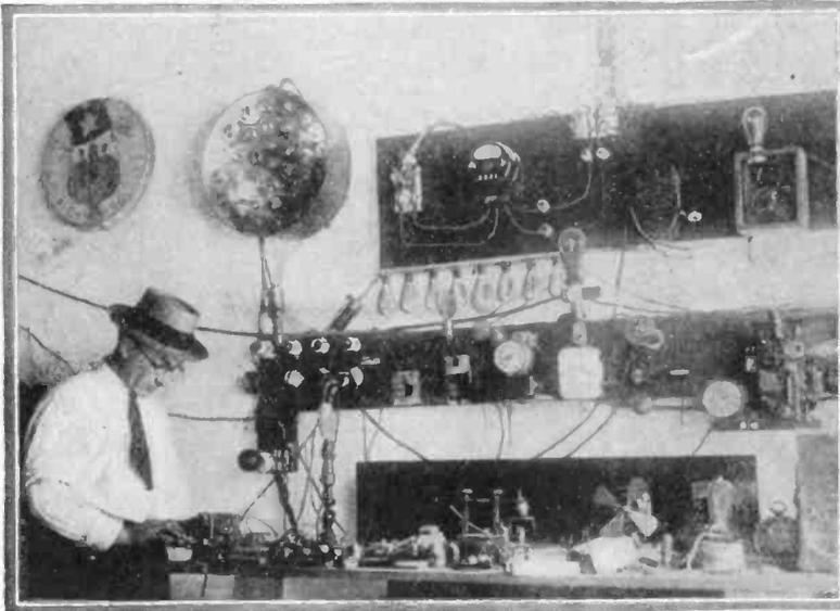
This may be called a telephone for the deaf, although it does not make any sound; by playing on a board like a keyboard on a typewriter attachment, lamps are lighted, a special one for each letter.
