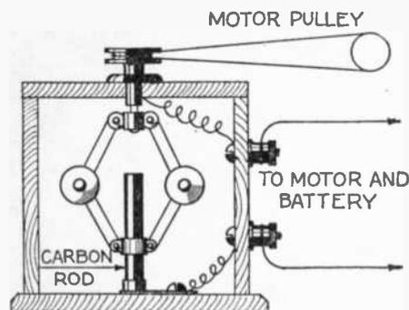
A centrifugal governor, varying the length of a carbon resistance connected in series with the electric motor. The motor turns the governor; practically constant speed is attained.
