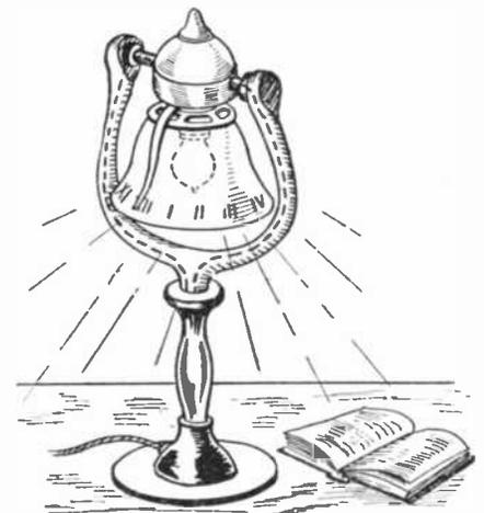
A very neat and useful electric table-lamp is illustrated above. The rim of the lamp reflector is graduated in hours and a pointer operated by a clock mechanism mounted above the lamp indicates the time. Though such clocks seem novel at the present time they were well known and much used during the 16th and 17th centuries.
