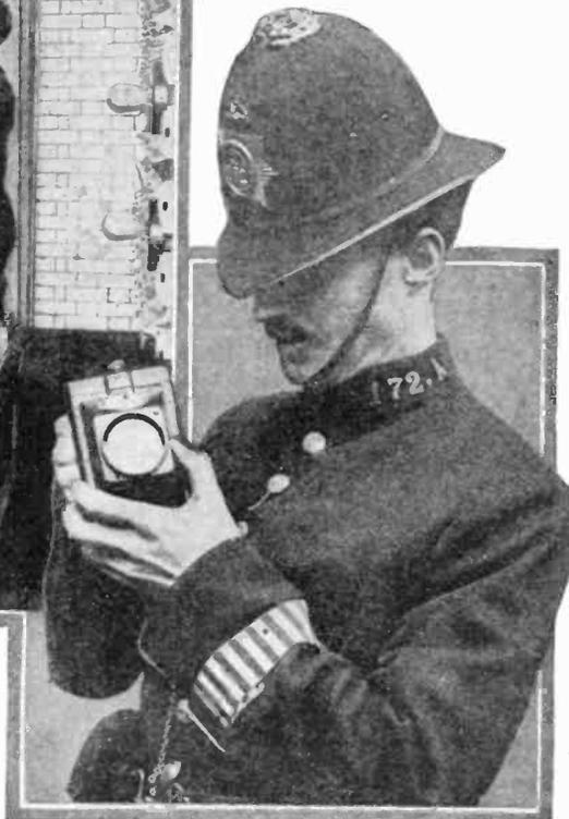
The London policemen have recently been provided with powerful flashlights that cast a strong beam over a distance of about 100 yards. The novel feature of these lanterns is the use of small storage batteries instead of the customary dry cells.
