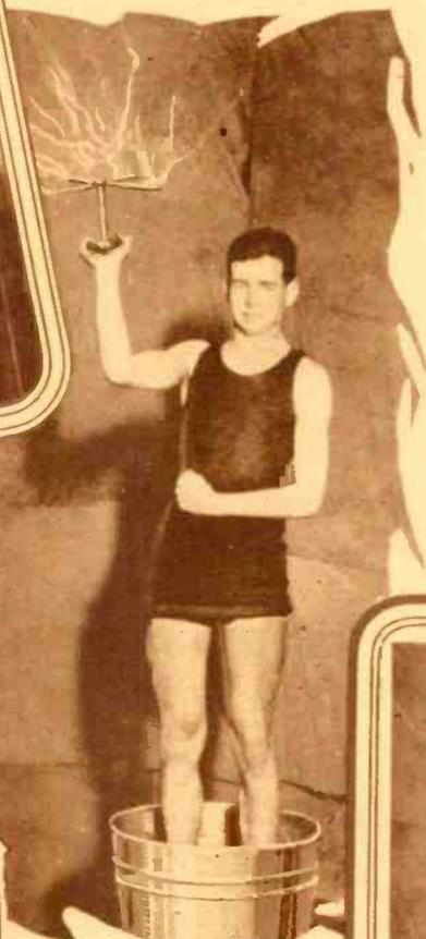
The sparks emitted by the arms of the small rotor at the left impart to it a spectacular motion. The Tesla coil is connected to the salt water bath in which the man stands.
