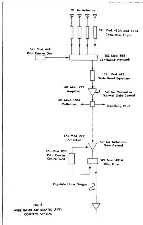
about twice as high at the upper end of the frequency band (Channel 13) as at the lower end (Channel 2). Moreover, this differential loss increases with temperature.
