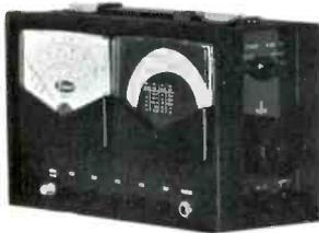
Dimensions: 5 1/4" x 11 1/4" x 7 3/4" □ Weight: only 10 lbs. including batteries □ Sensitivity: 5 microvolts minimum readable signal or 60 m/v full scale with sensitivity control at maximum □ Selectivity: all spurious responses including image more than 80 db down, 4.5 Mc/s or more away from selected frequency □ Battery Life: 180 hours continuous or better than 3 hours per week for one year.
