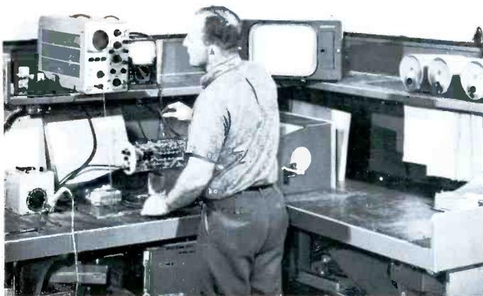
Camera test bench is another quality control point in the assembly of "Weather Channel."
