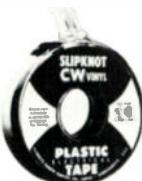
Similar to type #88. For waterproofing, taping splices, pin-holes, etc. Retains compliance even in coldest weather. 3/4 x 66" in Flip'n Cut Dispensers. Must be ordered in multiples of 12.
