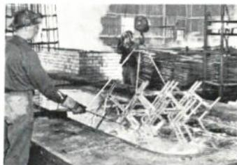
FINISHES Hot-dipped galvanizing after fabrication
