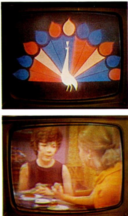
The color pictures above were received at the end of the 42-amplifier cascade in the Merced-Atwater mid-band tests.
