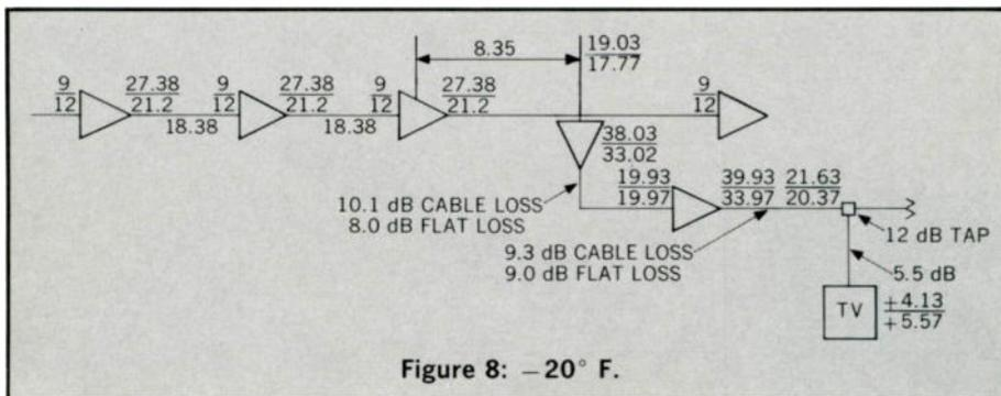
from +4.3 dB to +5.57 dB, swings of only 2.53 dB and 1.27 an improvement over normal AGC method of 12.2 dB at Channel 13. For the trunkline no output level specifications have been exceeded and inputs have remained constant so we can still cascade 80 amplifiers as our original planning had predicted. In fact when the temperature is below the maximum allowed in our design, 130°F, we have a built-in reserve for a safety factor. We won't attempt to work out the actual cascading of a normal
