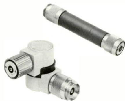
be twisted through 360°. When used together, these devices are engineered to permit movement in all three dimensions. Insertion loss of either of the new components is rated at less than 0.5 dB over a frequency range of dc to 12.4 GHz with SWR less than 1.1.
