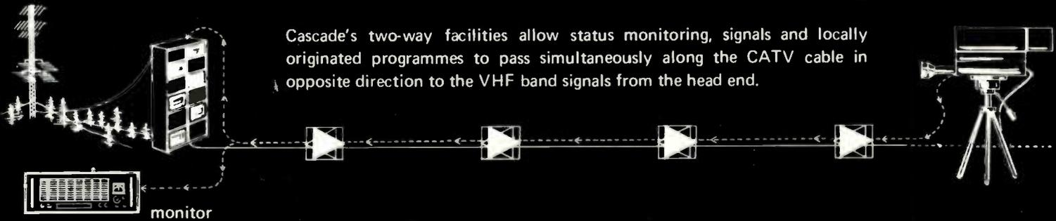
The output level of individual trunk amplifiers may be monitored constantly, day and night, at the head end or at any control point along a trunk line.
