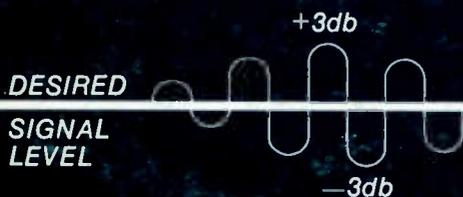
2. AGC circuit samples output signal, detects level changes and sends corresponding control voltage to reduce or increase Amplifier gain.
