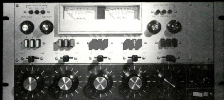
Run the program down the line while doing production work. The new A-16R dual channel audio console has five mixers handling three inputs each. The fifteen inputs have push-button selectors. A removable front panel is provided for custom needs. The A-16R uses only 8<sup>3</sup>/<sub>4</sub>" standard rack space or comes with handsome custom cabinet as an option. Learn how much more this console can do for you. \$995.
