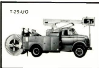
29' telescope model specially designed for self-supporting and CATV. Handles strand-wire medium cable.
