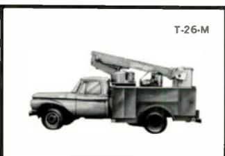
Long 26' reach on small vehicle. Easy bucket access. Built-in electric power. Capacity 300 lbs. for transfer and reconstruction.
