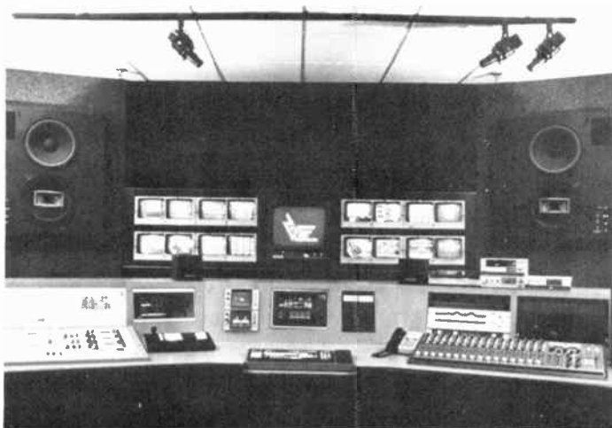
Caesar Video one-inch editing suite with CMX-340X, GVG 300-3A, three VPR 3s, BVH-2000, ADO, two Dubners two Chryons, two Paint Boxes and VAS IV controller. The equipment also features a Quantel Harry DCR-7700 realtime digital cel recorder, installed by Caesar in what the company calls the nation's first digital animation studio.
