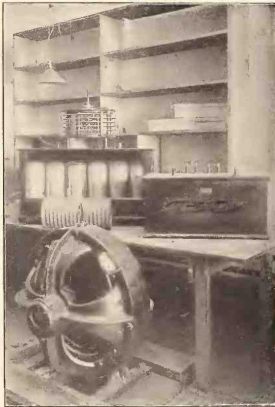
GENERATING PLANT FOR THE WIRELESS TELEPHONE.
