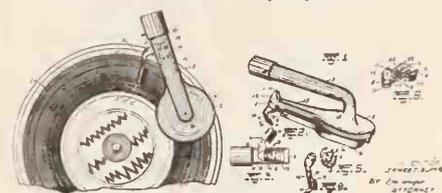
said reproducer and attachment; Fig. 3 is a broken bottom plan view thereof; Fig. 4 is a perspective view of the attachment detached; Fig. 5 is a broken perspective view of the reproducer arm; Fig. 6 is a broken perspective view showing a modification.
