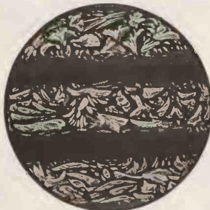
No. 3—One-thirtieth inch of record surface magnified, with the three grooves occupied by glistening products developed by an invisible portion of a drop of water.
