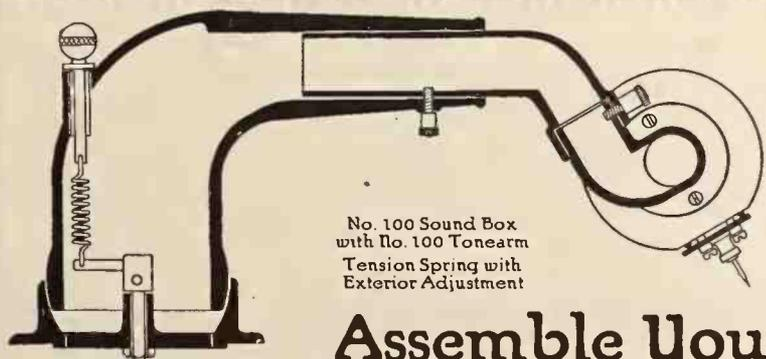
No. 100 Sound Box with No. 100 Tonearm Tension Spring with Exterior Adjustment
