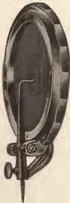
**OUR MAGNETIC REPRODUCER:** Produces pure tone qualities and wonderful volume. The method of constructing the reproducer and the pivotal arrangement of the stylus bar allow the vibrations to pass without interruption from the needle to the diaphragm. The magnetic attraction of the needle arm gives an outward strain on the diaphragm, making it more sensitive to vibration influences.
