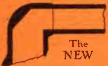
That same angle turn with the solid inclined plane deflecting the sound waves straight downward into amplifying chamber. That same famous Scotford tone—the tone of refinement—genuinely musical. Now in a tonearm of accepted, conventional, popular design. WRITE FOR SAMPLES.
