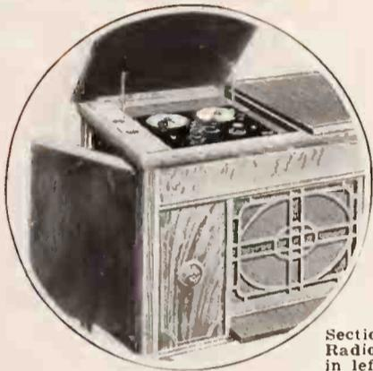
Sectional view of cabinet showing Radiola Super-Heterodyne installation in left-hand top convenient to operation. (Phonograph equipment available on right-hand top side of cabinet.) No outside wires required. Large directional loop has been installed in swinging left-hand END PANEL of cabinet.
