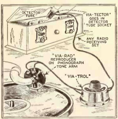
This illustration shows the units and connections of the Via-Rad reproducer and the simplicity of the entire arrangement.
