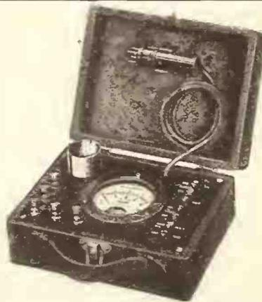
Pattern No. 133 Radio Set Analyzer.—Grid, plate and filament conditions of all tubes in a radio set can be quickly analyzed. Separate terminals provide for making circuit tests with the instrument used either as a high resistance voltmeter or as a milliammeter. Scale ranges are 0-8-80-200 volts and 0-20 milliamperes.
