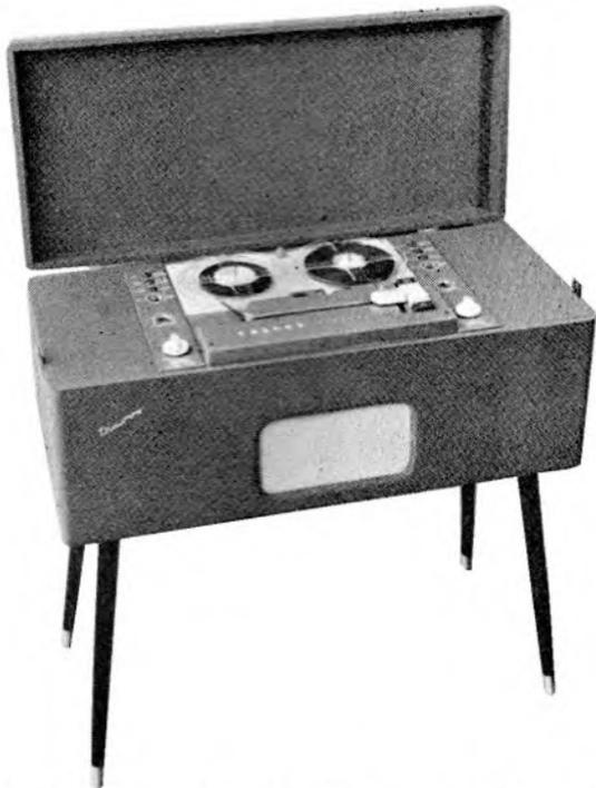
*This handsome cabinet has been custom-built to house the Truvox Mk IV deck, Type K stereo amplifier and a speaker for monaural playback*
