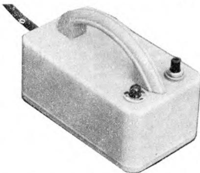
for complete erasure of the tape. Like its smaller version, the Mk 2 may also be used to de-magnetise tape heads.
