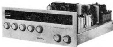
and Foster Seeley discriminator, which provides a sensitivity of 1.5 mV and has twin variable outputs for future stereo radio. Tuning is by meter.
