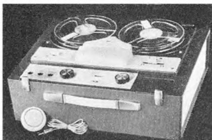
eye recording level indicator, combined tone control, and an extension speaker socket (3-5 ohms). The built-in loudspeaker, a 7 x 3½ inch unit, handles an output of two watts.
