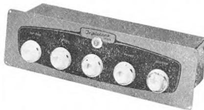
treble control from  $+18$  dB to  $-18$  dB at 10,000 cps. The tape output is 500 mV into 100 K ohms  $\pm 1$  dB 30-20,000 cps.
