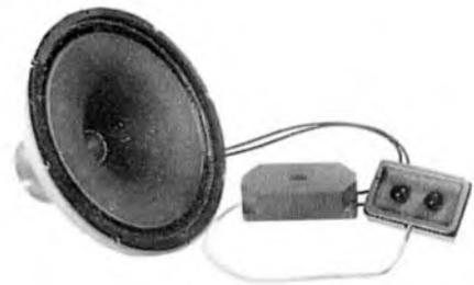
Impedance is now 8 ohms, making the unit particularly suitable for all types of transistorised amplifiers. The mass of the LF diaphragm assembly has been increased to improve bass response in small enclosures. The improvement at the lower end is said to be approximately half an octave down for a given size enclosure relative to the older units.
