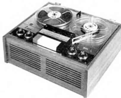
Each machine has two acoustically matched loudspeakers size 7 x 4 inches built-in, and the claimed frequency response is from 30 to 17,000 Hertz plus or minus 3 dB at 7½ ips. Signal-to-noise ratio is claimed as better than 48 dB on the R 52, 46 dB on the R 54. Equalisation is to the new CCR standard and outputs are provided at external speaker sockets to give 6 watts into 8 ohms.
